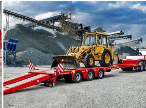
**Dimensions:** Length: 13190mm \ Width: 2550mm extendible to 6000mm \ Gooseneck length: 3950mm \ Chassis height from ground: 890 mm \ Loading deck length: 9240 mm extendible to 6000mm
