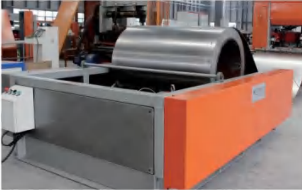
7吨地辊开料架 7TRoller type decoiler
