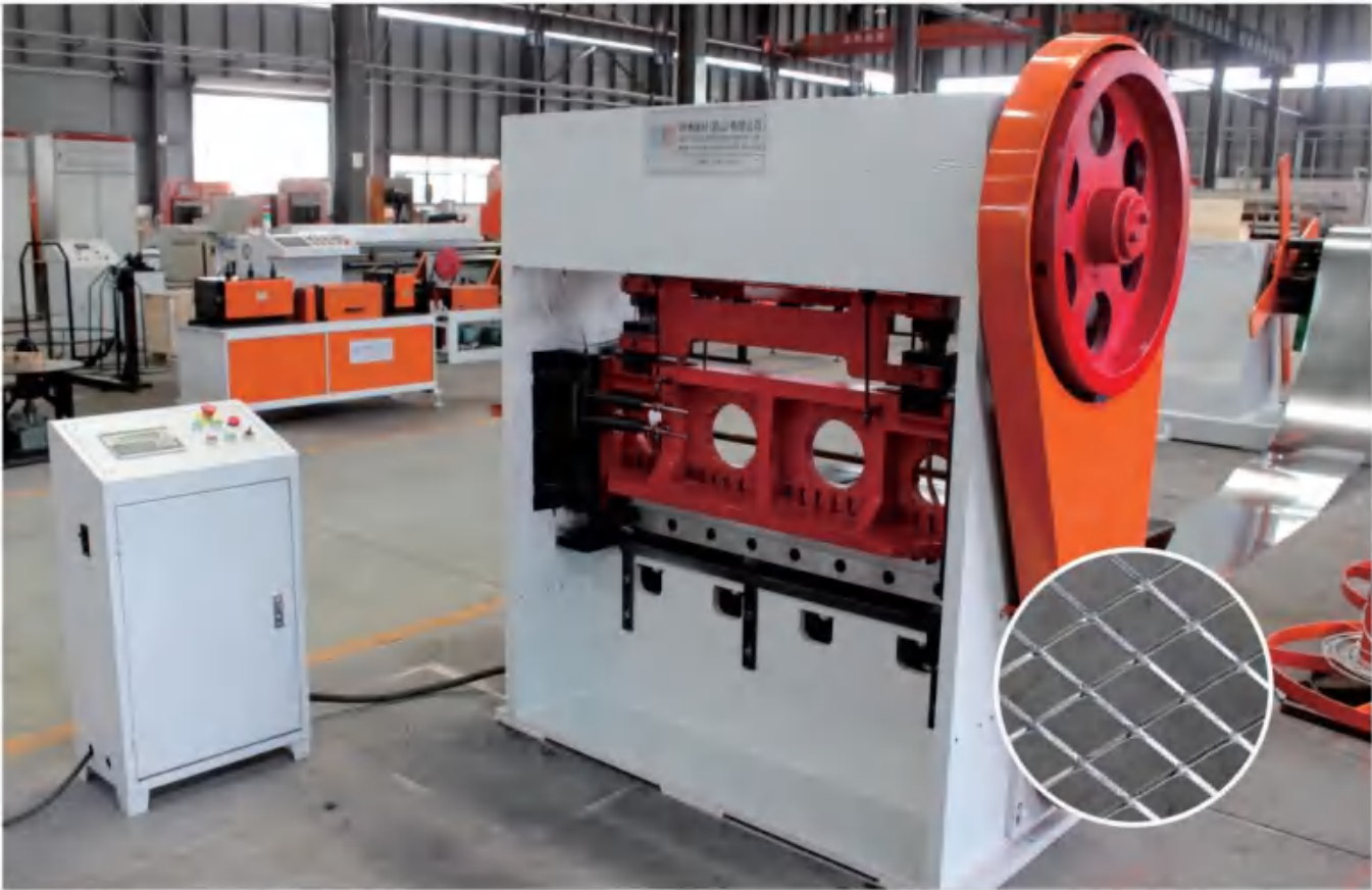
ABE-1.0-1000 (16T) 钢板网机 / Expanded Mesh Machine
