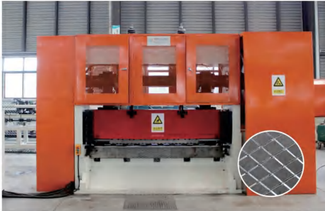
ABE-6.0-1600 (100T) 钢板网机 / Expanded Mesh Machine
