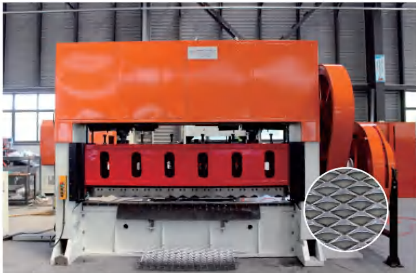
ABE-6.0-3200 (160T)钢板网机 / Expanded Mesh Machine
