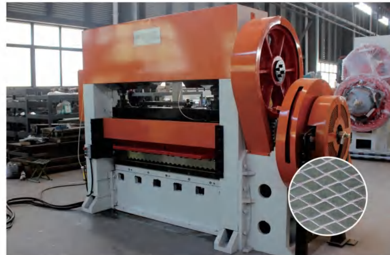
ABE-2.5-1500 (40T) 钢板网机 / Expanded Mesh Machine
