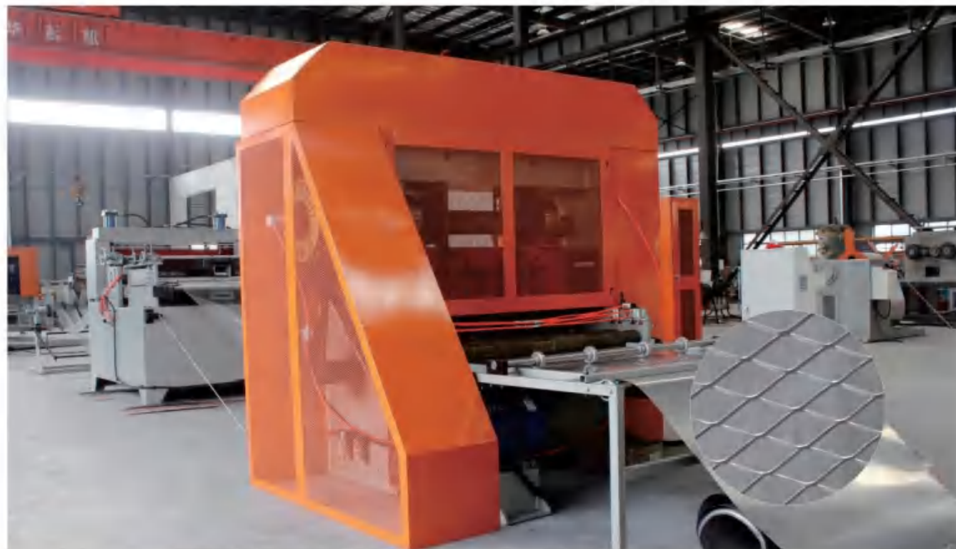
ABE-GS40-1250 40T)高速钢板网机/ High Speed Expanded Mesh Machine
