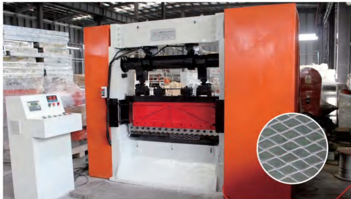
ABE-4.0-1300 (60T) 钢板网机 / Expanded Mesh Machine
