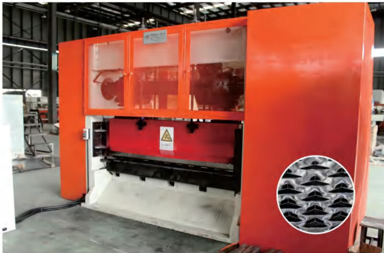
ABE-6.0-2000 (100T)钢板网机 / Expanded Mesh Machine
